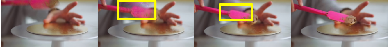
Figure 25: An example where GRACE performs poorly. It shows four consecutive decoded frames where the pink brush moves down quickly. Some artifacts in The yellow box degrade the frame quality and impact the SSIM.
